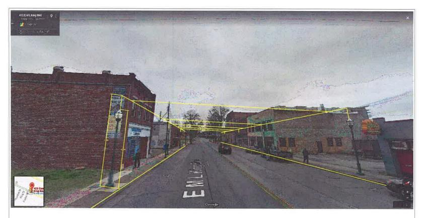
Layout lines estimate the lowest point of eighteen(18) feet above the roadway. Douglas St traffic signal does not appear to be obstructed at this lowest point.
